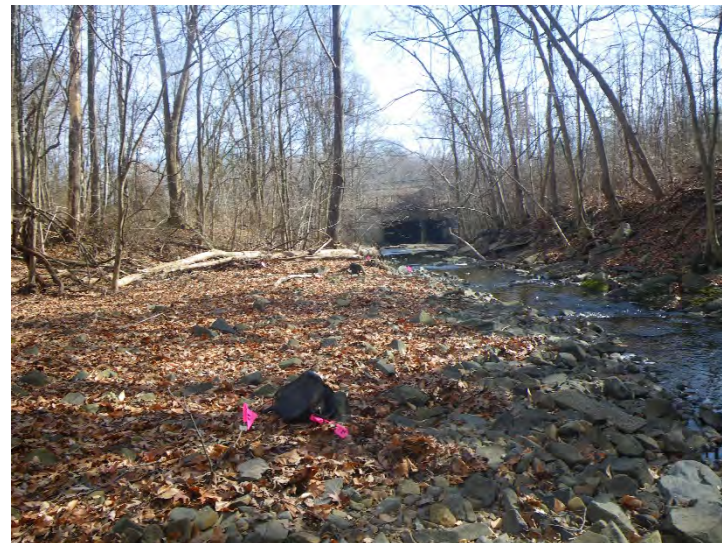
Facing downstream at cross section Sta. 12+03 (note flagged bankfull stage along point bar)
