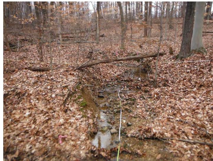
Facing upstream from Sta. 6+30 at surveyed cross section. (point bar feature to the right of the tape in the photo associated with bankfull stage).
